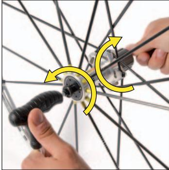
Insert a 5 mm Allen wrench into each end of the axle and unscrew the axle end screw on the drive side.
