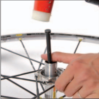
Extract the bearings using bearing press kit M40120.
