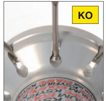
Screw each nipple uniformly (1 turn of the spoke wrench for each spoke and for each turn of the wheel) to tension the wheel, checking the heads are correctly positioned in the groove of the hub to ensure a spoke does not become unhooked and to prevent the hub from breaking.
