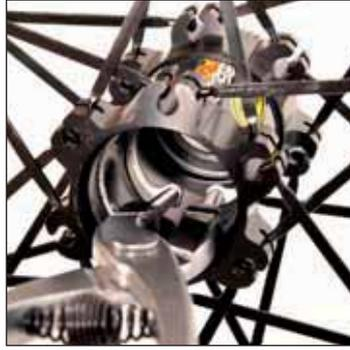
From the non-disc side, using an interior circlip pliers, refit the second interior circlip (disc side) in its groove, followed by the first interior circlip (non-disc side) in its groove.
