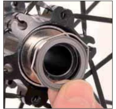
Mount the pin / washer assembly on the non-disc side by presenting the conical part toward the inside, and the grooved part toward the outside.
