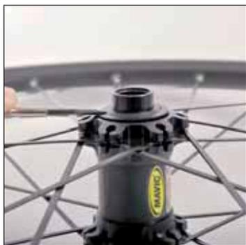
Remove the dust cover from the non-disc side:
