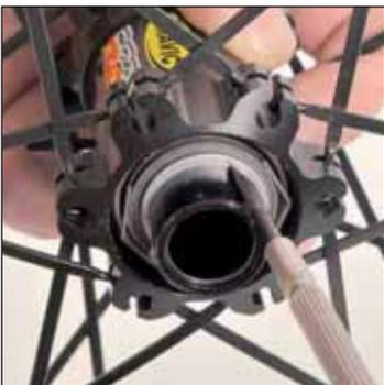
Using an external circlip pliers, replace the external circlip on the axle, non-disc side. Make sure that the circlip is correctly positioned in its groove by pressing on 3 points.
