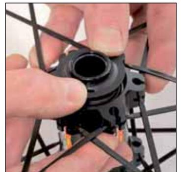
Replace the dust cover by pushing it parallel to the axle.
