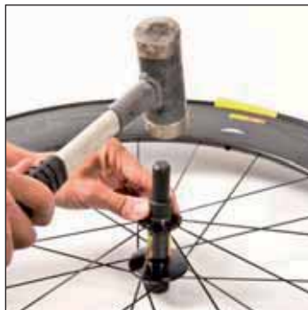
Fit the new ORL bearing with M40120
